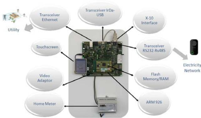
Figure 3- Hardware architecture of the ERG
