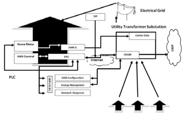
Figure 1- Smart Grids Architecture
